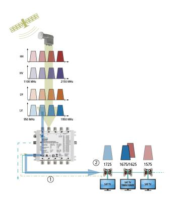
The receiver uses special DiSEqC commands with its user band ID to tell the converter (1) which program (i. e. which polarization and which center frequency of the desired satellite transponder) the single cable converter must put into the assigned user band of the receiver (2).
