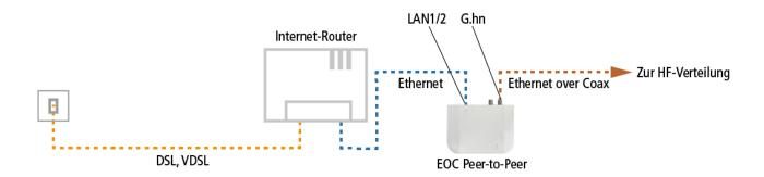
The connection to the Internet is established in the example with the help of the Internet router via DSL or VDSL. The EOC modem is connected to the Internet router via an Ethernet cable at the LAN1 or LAN2 port. The G.hn port of the EOC is connected to the RF distribution using a coaxial cable with F connectors.
