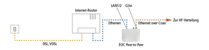
The connection to the Internet is established in the example with the help of the Internet router via DSL or VDSL. The EOC modem is connected to the Internet router via an Ethernet cable at the LAN1 or LAN2 port. The G.hn port of the EOC is connected to the RF distribution using a coaxial cable with F connectors.
