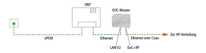
The connection to the Internet is established via optical fibre with the help of the ONT. The EOC is connected to the ONT (Optical Network Termination) via an Ethernet cable.
