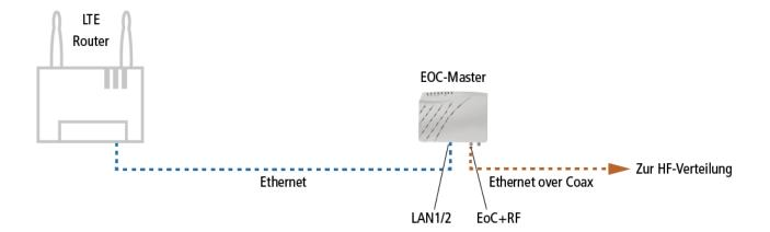
The connection to the Internet is established via cellular networks with the help of the LTE router. The EOC is connected to the LTE router via an Ethernet cable.
